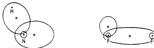
Figure 2. Intersection between the xy plane and selected charge ellipsoids of \text{H}_3\text{N}\cdot\text{F}_2 . The hydrogen nuclei of \text{NH}_3 are rotated to eclipsed configuration with respect to the lone pair ellipsoids of the electron pair accepting fluorine nucleus; otherwise, the geometry is equal to the equilibrium geometry as determined in this work. Charge centroids are marked with a cross (X) and nuclear positions with a dot (●). (The xy plane is defined by the nitrogen nucleus, a halogen, and a hydrogen nucleus.)
